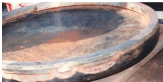
Disc of a swing check valve that has been corroded by seawater
